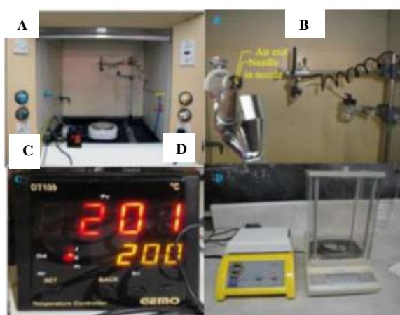
Fig. 2 A: experimental set up of the spray pyrolysis deposition SPD. B: Air atomizer. C: Gemo DT109 temperature controller, and D: Digital balance with the magnetic stirrer.
